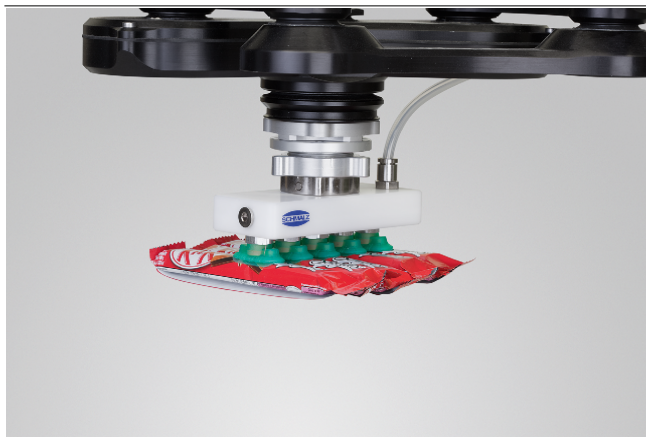
Bellows suction cups SPOB1f when handling small flow-wrap packaging
